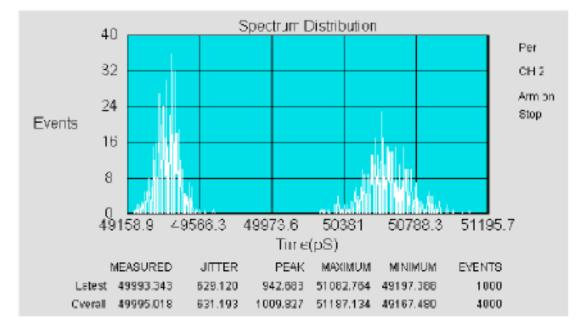
Plot is a period histogram of the 2XQ output of an off the shelf PLL. Input frequency is 10MHz; Output frequency is 20MHz, or 50ns period. Measurement is done automatically without external arming. Sample size = 1000.
