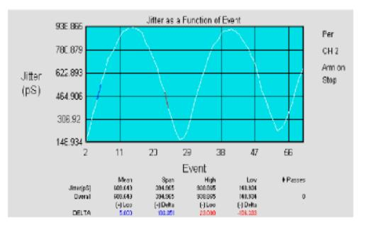
Plot shows jitter accumulation on the 2XQ output of an off-the-shelf PLL. Input frequency equals 20MHz; Output frequency is 40MHz. Plot shows jitter buildup over 28 consecutive cycles.
